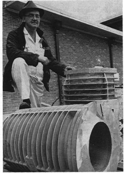
LAYOUT OPERATOR CHARLES RILEY stands by finished castings of new wind tunnel pieces. The units will now move into the Development Shops for final machining. Thin "ribs" on the outside of the casting represent a foundry achievement.
